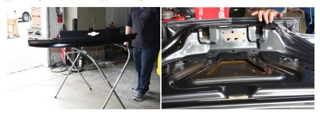
**Step 2**: Flip the trunk over so that you can see how the current spoiler sits on the old trunk. This will give you an idea of how the spoiler will sit on the new trunk. In our case, we noticed that there are small gaps at the bottom of the spoiler. We will expect to see similar gaps with the new trunk.
