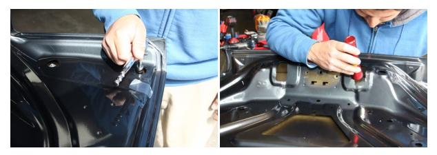
**Step 5:** Once you have confirmed that all of the screws have been removed, carefully pull the spoiler down to remove it. A partner can help you hold the other end of trunk so that you do not drop it while taking the spoiler off.
