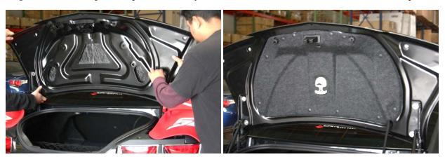
**Step 19:** If applicable, reinstall the trunk plugs removed in Step 3.
