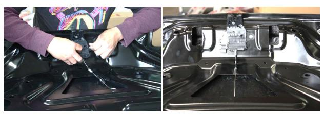
Step 18: With the help from a partner, install your Seibon Carbon trunk. Reinstall trunk cover, clips, etc..
