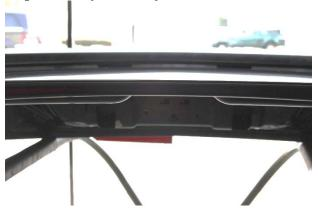
**Step 16:** Carefully flip the trunk over so that you can reinstall the screws on the spoiler. It may be necessary to create or enlarge a few holes on the inside of the trunk so that you can tighten up the spoiler's screws.
