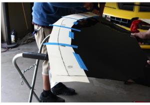
**Step 9:** Important: make sure that you have test fitted the Seibon carbon trunk before drilling spoiler mounting holes as described in the following steps, especially if this is a newly purchased trunk.
